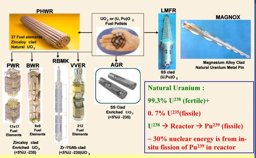
LWRs & PHWRs account for more than 90% of operating nuclear power reactors. They use low enriched uranium (<5% U<sup>235</sup>) and natural uranium respectively as fuel in the form of uranium oxide pellets encapsulated in zirconium alloy cladding tubes
